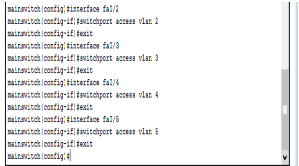
Figure3. Assigning Ports in Main Switch
