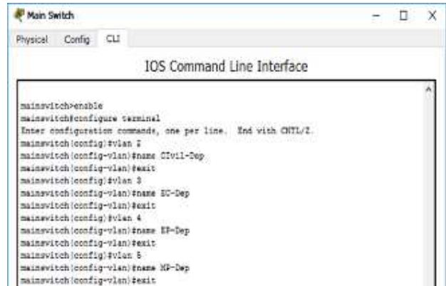
Figure2. Creating VLAN in Main Switch
