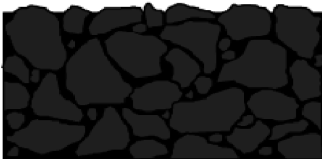
Fig.1.1 Gap Graded Mix Structure
