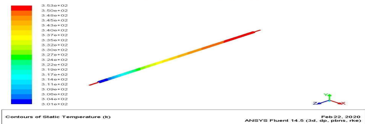
Figure3. Contours of static Temperature for Cu-Al 2 O 3 /Water based hybrid nanofluid of 0.3% volume concentration at 0.2 litre/min flow rate.
