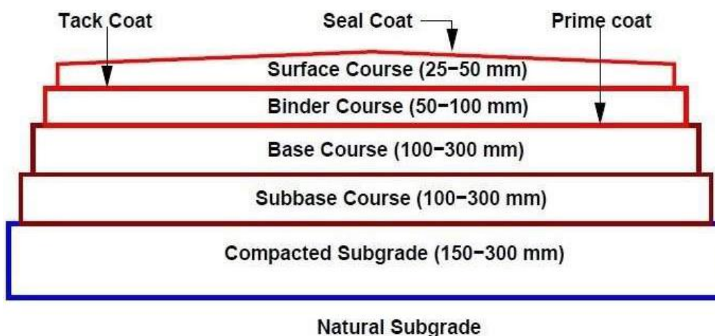
Fig 1 Typical cross section of a flexible pavement
