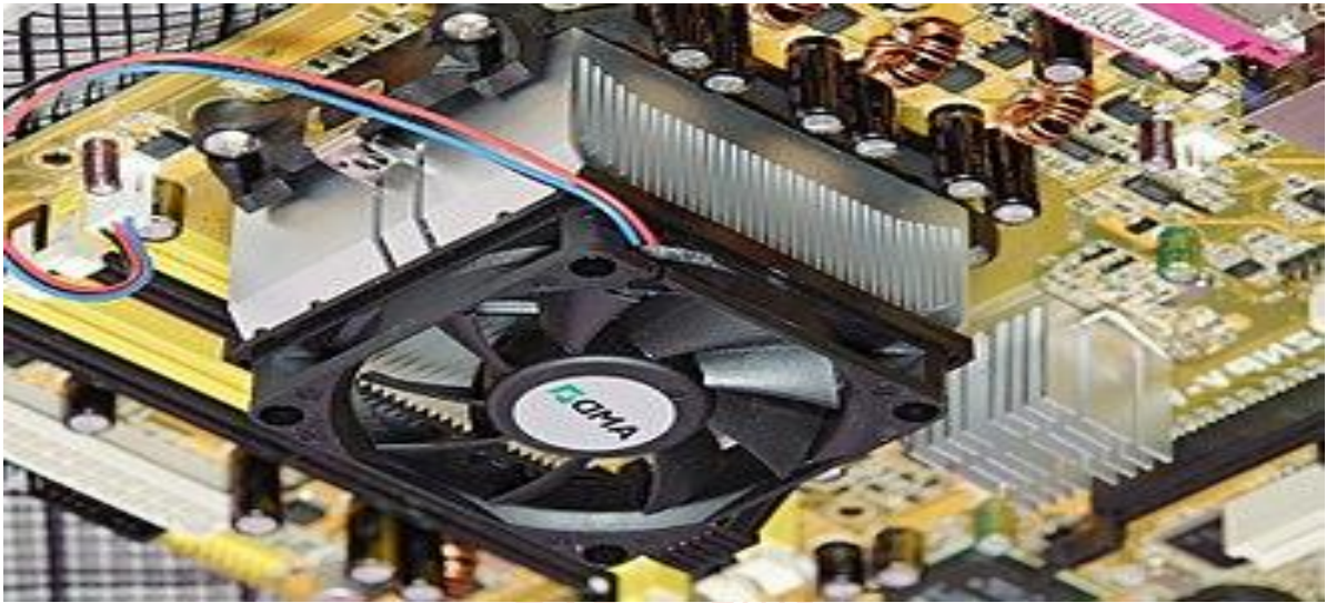
Figure 2: A fan-cooled heat sink on the processor of a personal computer.
