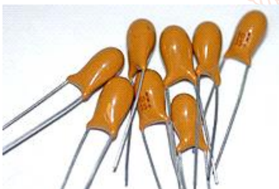
Figure-9: Solid-body, resin-dipped 10 μF 35 V tantalum capacitors. The + sign indicates the positive lead.
