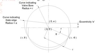
Let the valve bore be indicated by a circle of radius 'r' with its centre at the origin. Equation of the circle is given by.
