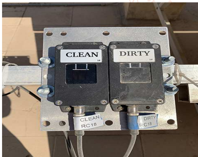
Two sensors in the field show the difference between one that is regularly cleaned and one that never is. Photo by Matthew Muller, NREL
