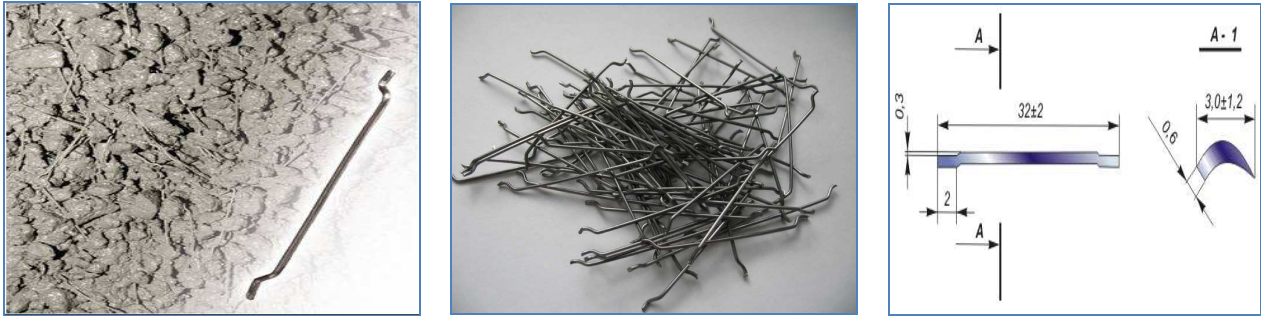
Fig. 1 Type of steel fiber.
