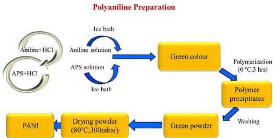
Fig.5. Formation of PANI thin film
