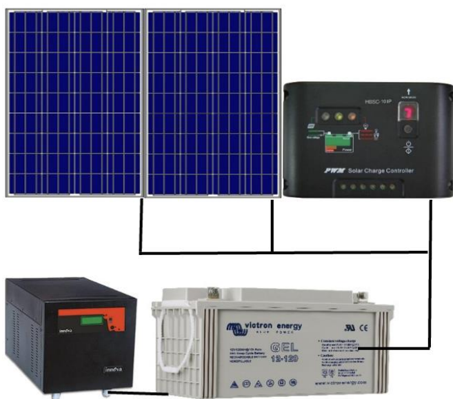
Figure 2.0: The Assembly of the Solar Photovoltaic System.( Battery University ,2010).
