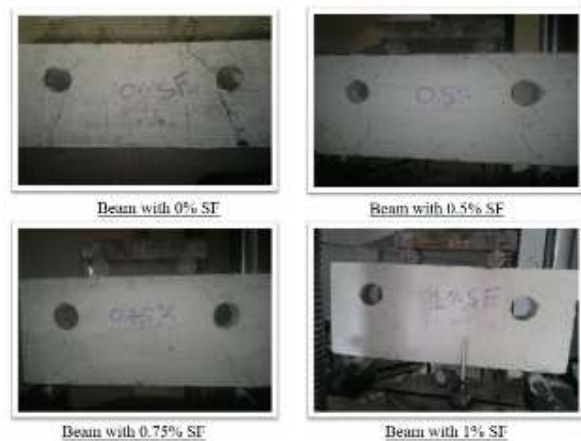
Fig. 8 Failure of deep beam with web opening at position A
