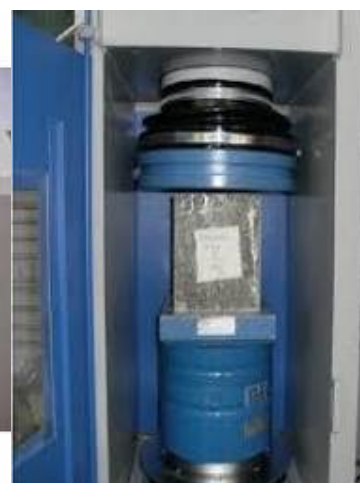
CONCRETE SPECIMEN ON COMPRESSIVE STRENGTH TESTING MACHINE & TESTING CUBE FAILURE
