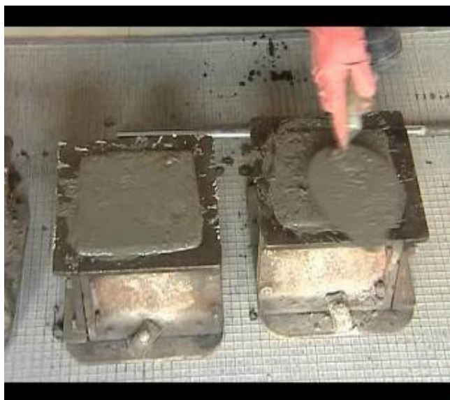
Compressive strength test15
