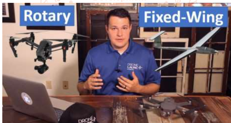
Figure 1 Fixed-wing and rotary types of drones [1].
