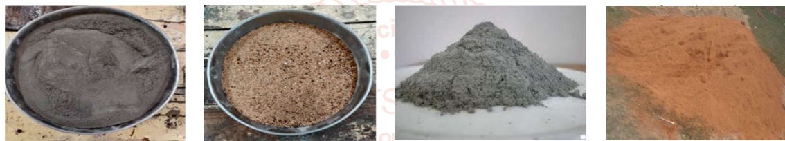
Figure 3: Materials Used a) Cement b) Fine Aggregate c) Fly Ash d) Surkhi
