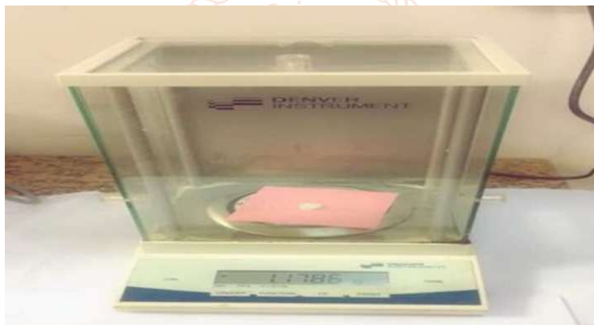
Figure 2.3. Four digits sensitive balance used for weight variation of different types of paracetamol tablets.
